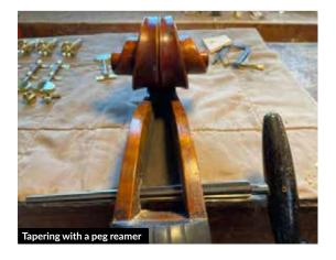
Then I use two different peg reamers: a straight cello reamer, tapered at 1/25 with a maximum diameter of 16mm, and the same sized brass spiral reamer to finish the job. Also, since the tuner's maximum diameter is 16mm, I know exactly when to stop – at the end of the reamer! After the first peg is fitted I do the E string, and work my way up to the A, and finally the D string.
