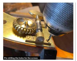
6 I make the tuner holes using a knife made of very hard Tyrolean steel, which makes it easier to cut the softer brass. Then I finish the chamfer of the plate, firstly with a fine metal file and then with sandpaper. Finally I polish the plate until no toolmarks can be seen.
