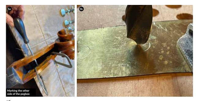
5 Once they fit, I fix the plates with two clamps on the outside wall and mark the outline of the pegholes – with a pointed drill bit – from the opposite pegholes (5a). Taking the clamps off, I make a circle to mark the middle of the hole to be drilled (5b).
